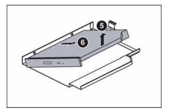
**9** Unscrew the two screws (5) holding the optical drive interface board on the back of the optical drive, then remove the interface board.
